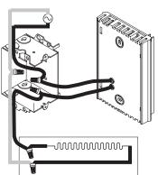
Install the base onto an electrical box.
